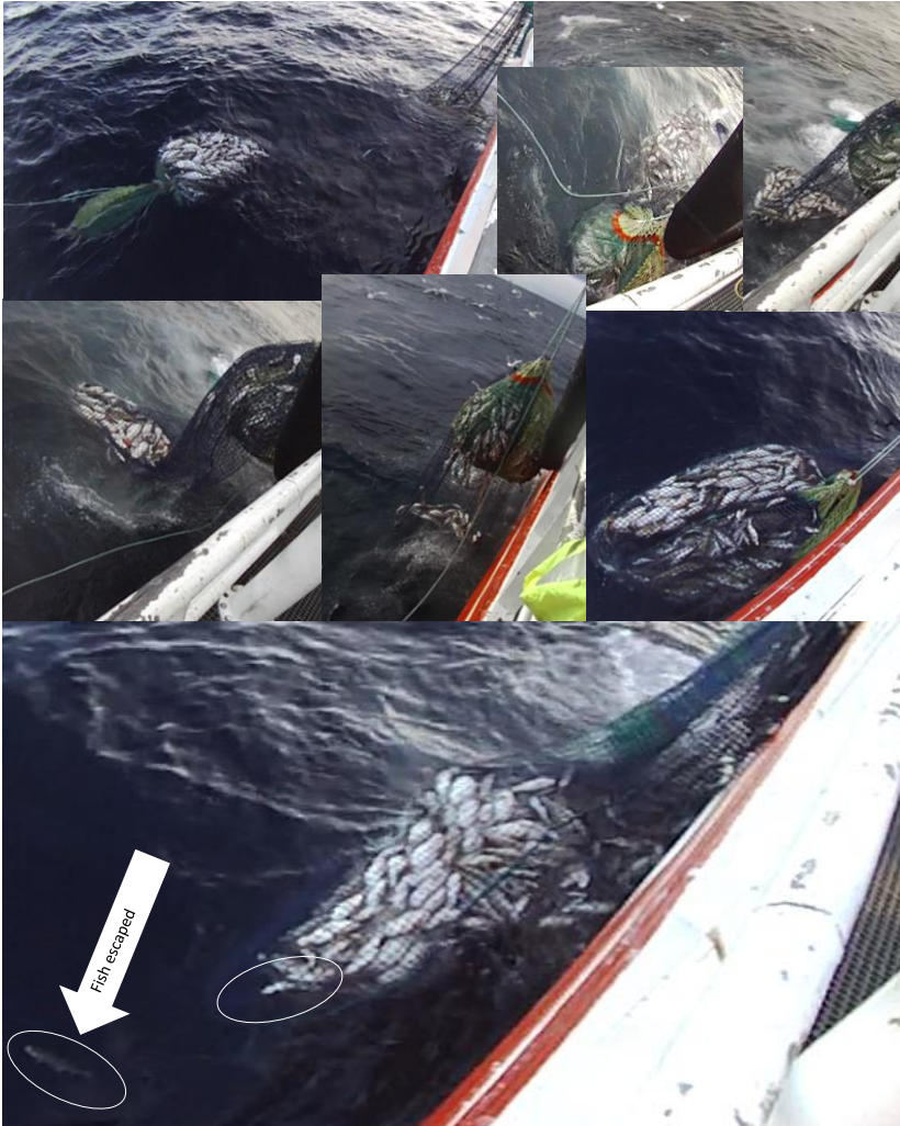
Fig. 3: Collage of photos taken during the "sacking" operation. The photos show how the fish-lift is operated by releasing part of the catch into it while the remaining part of the catch is kept in the square mesh section of the codend at the surface. Several of the photos show that the catch remaining in the square mesh section is surrounded by tensionless square meshes. Further, there is evidence that escapement at the surface does occur.
